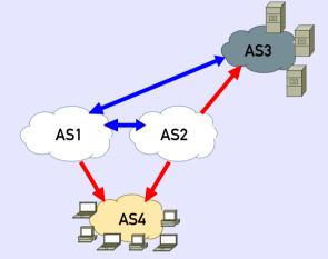
We have to fix the redundancy. This can be achieved by the additional advertisement of the less-specific /13 and /16 networks towards AS1 and AS2, additionally to the ten /17 more-specifics, which are advertised 50:50 to either AS1 and AS2.
