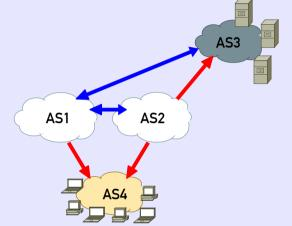
Ok, selective advertisement has drawbacks, but there is a workaround. The traffic from AS3 must be distributed over both transit links. I'm going to de-aggregate the /13 and the /16 into ten /17 and advertise five to each AS1 and AS2.
