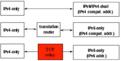
As yet undefined/unimplemented Magic (TCP relay could be SSH tunnel)
